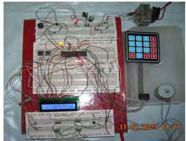
Fig. 11 Experimental testing of the door access control system
